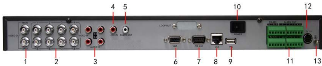
Figure 16. DSR-805-h Rear Panel
