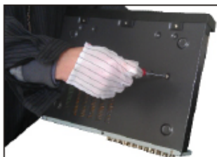
5.Fix the screws of the hard disk.
