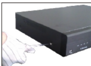
1.Tear down the fixed screws of the device top cover .
